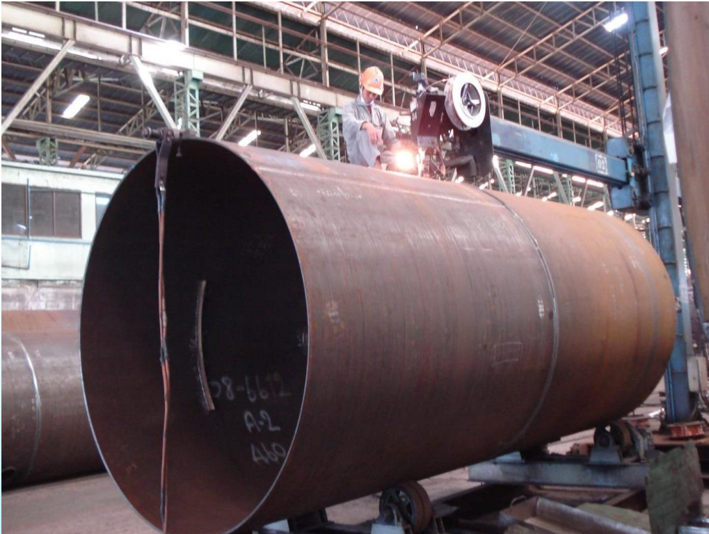
Semi-Automatic Longitudinal Welding with Manipulator
