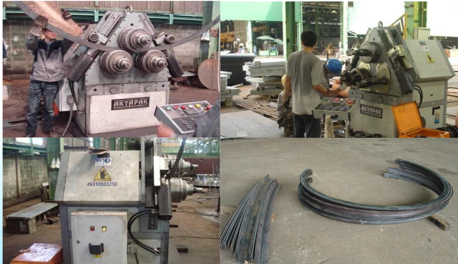
NC Hydraulic Profile Bending Machine: Max FB 100 x 25t x 800r
