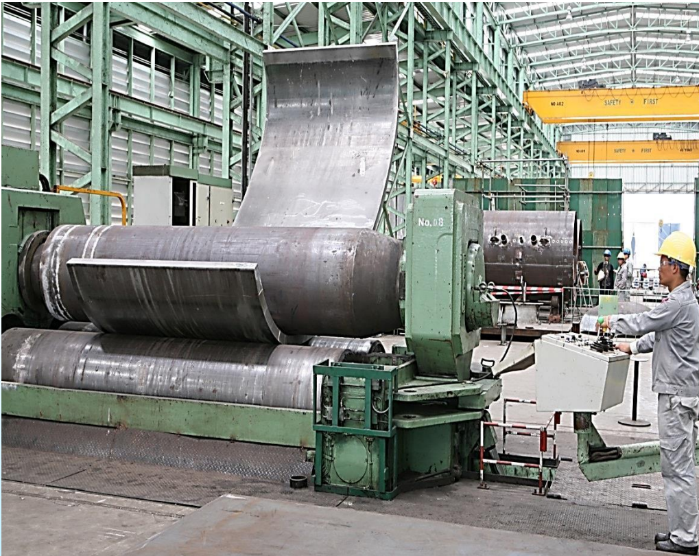
Plate bending: Capacity: 125 mm. (5") x 3,675 mm Width.
