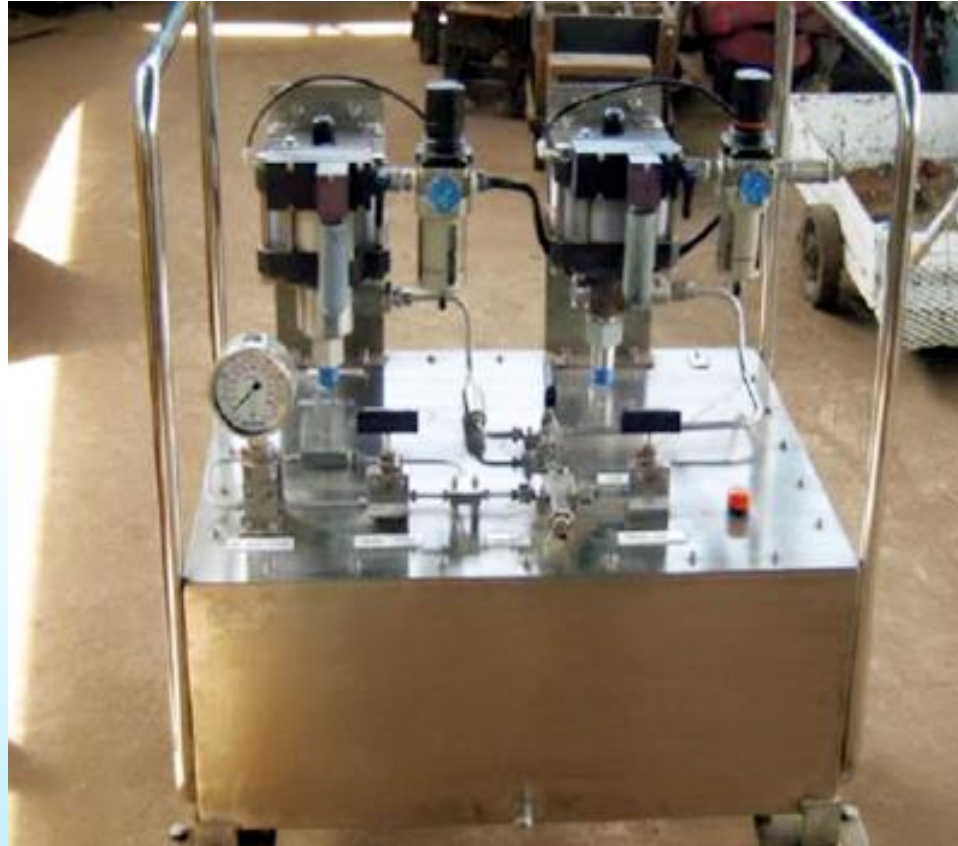
High Pressure Test Pump - Output (max) 10,000 psi Flow (max) 668 sq. inch
