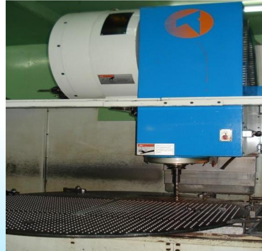
Specification: 1 M Wide x 3 M Long x 300 mm Thickness capability
